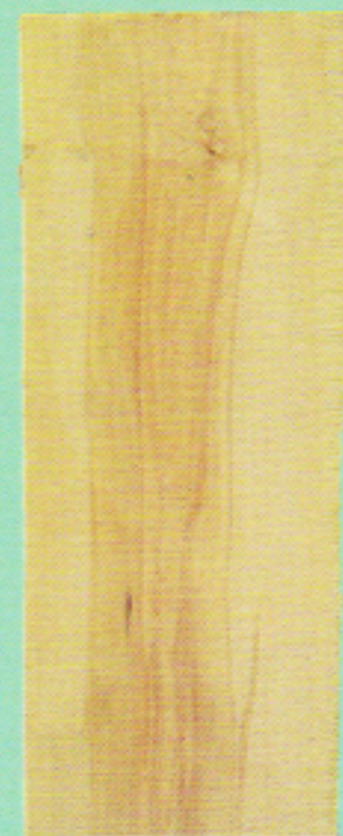
◀ Not acceptable in white wood
